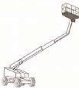
of an elevated lift are on a solid base. Use outriggers, if provided. Set the brakes and use wheel chocks when on an incline. Do not exceed the load limits of the equipment. Allow for the combined weight of the worker(s), tools and materials.
